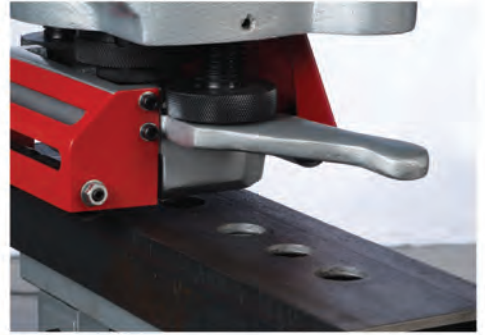
Punching Channel Flangers and Angles
