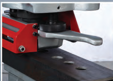
Punching channel flanges and angles
