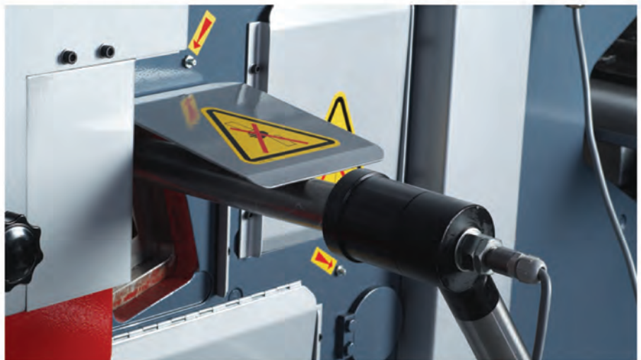
Touch and cut electrical back gauge
