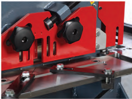
7 3/4" x 19/32" & 11 3/4" x 1/2" Flat steel cutting capacity.
