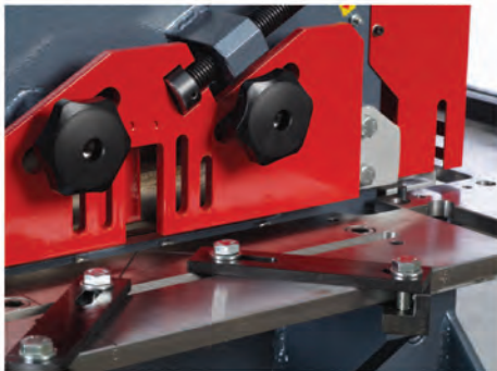
This station allows the miter cutting of angle iron (horizontal leg).
