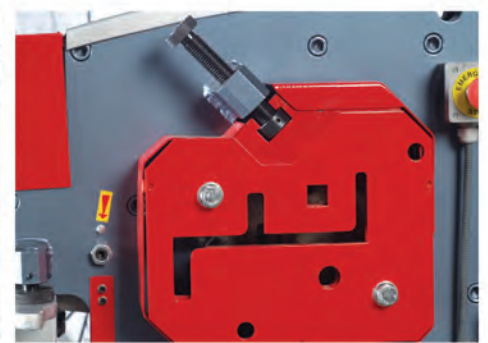
Angle shear station with Z shape apparatus. With this it is possible to make miter shears on angle bars.
