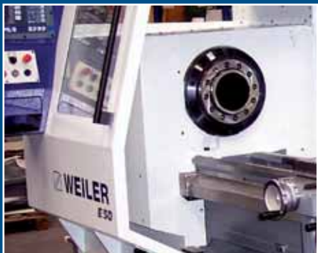
Version with 6.5 inches spindle bore
