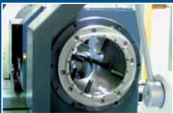
Ring steady rest with 10.6 inches diameter
