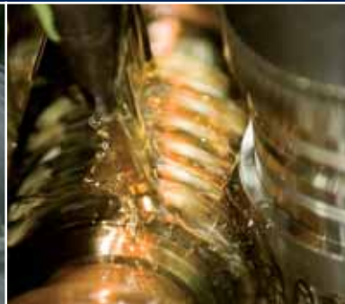
Gear wheel production / hobbing
