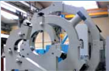
Steady rests for diameters up to 57 inches
