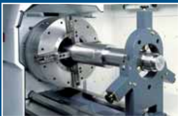
Pneumatically actuated front-end chuck with fixed rest
