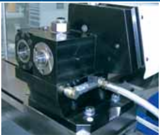
Tool holder head for turning, drilling and milling
