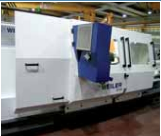
Version with additional sliding cover and splash guard
