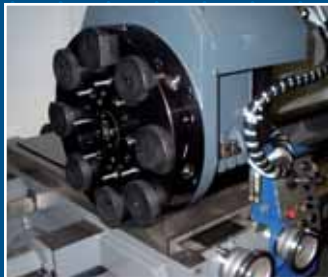
8 station disk turret with driven tools, 1.6 inch shank diameter
