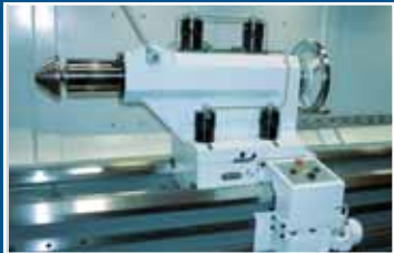
Tailstock with automated clamping and dedicated drive
