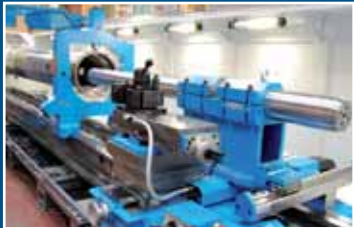
Heavy-duty boring bar holder with additional support and 6.3 inches bore
