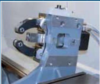
Travelling, self-centering rest, hydraulically actuated
