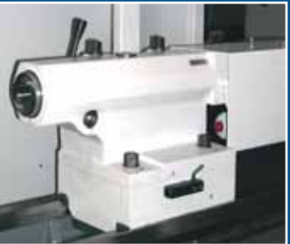
Tailstock with hydraulically actuated quill
