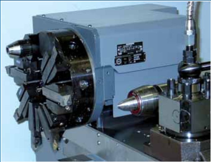
8 station disk turret with / without tool drive
