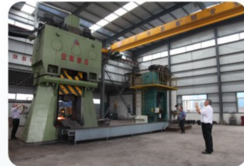
125KJ数控锤在安阳联达精锻锻造盆角齿 125KJ CNC hammer forge bevel gear in Lianda
