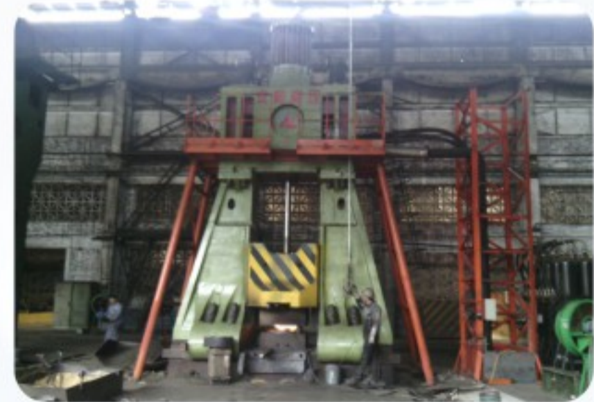
18T全液压模锻锤锻造轮船连杆 18T fully hydraulic closed die hammer forge vessel connecting rods
