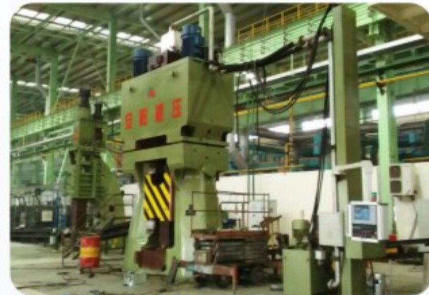
国内首台160KJ数控锤湖州锻造法兰 160KJ CNC hammer forge flange in Huzhou
