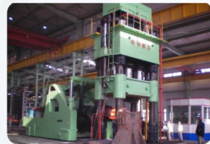
3150T自由锻液压机和20T操作机在本溪客户 3150T open die forging press and 20T manipulator in Benxi
