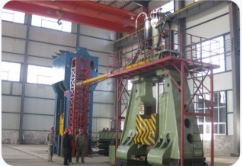
16T液压模锻锤锻造铁路锻件 16T hydraulic closed die hammer forge railway parts
