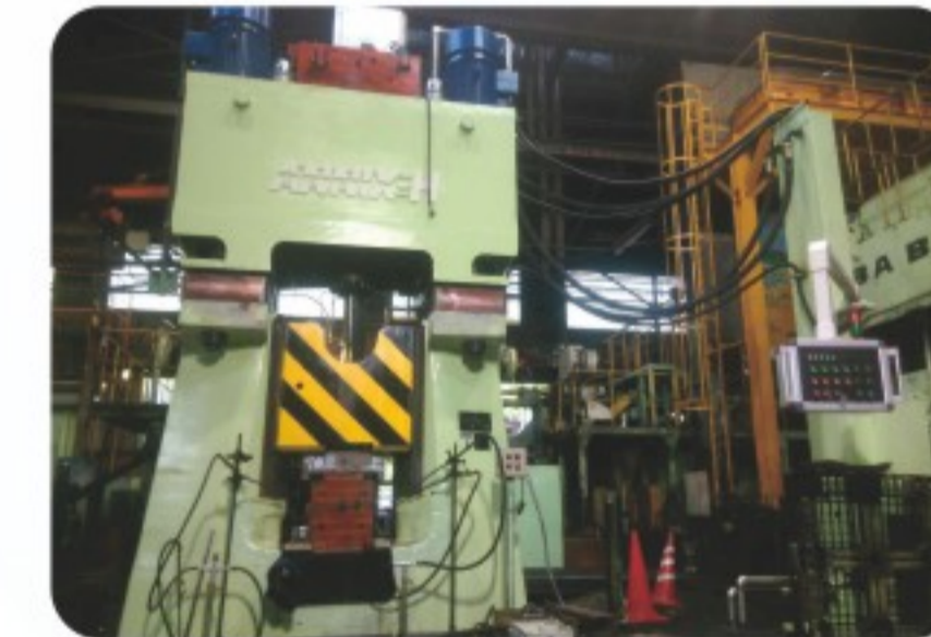
63KJ数控锤在日本锻造连杆 63KJ CNC hammer forge connecting rod in Japan
