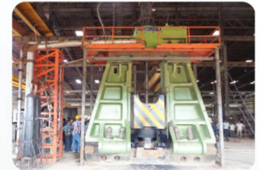
10T电液模锻锤出口印度锻造高颈法兰 10T hydraulic closed die hammer forge flange in India
