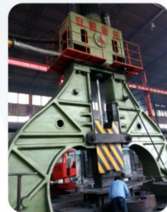
8T全液压自由锻锤锻造风电锻件 8T fully hydraulic open die hammer forge wind power forgings
