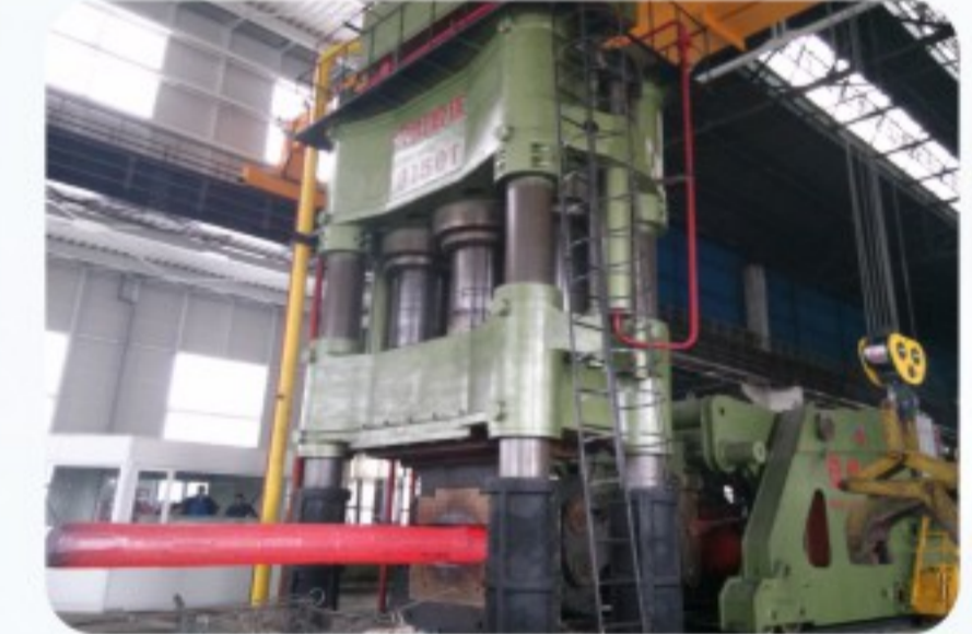
3150T自由锻液压机和 30T数控锻造操作机在罗马尼亚 3150T hydraulic forging press and 30T manipulator in Romania
