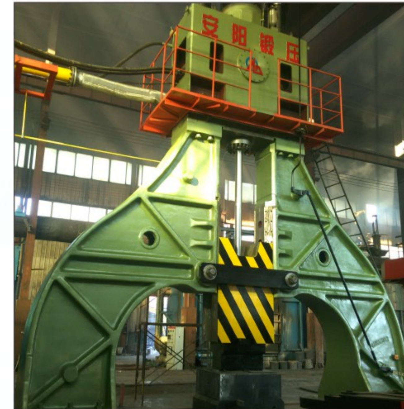
(注: 我公司可以对旧自由锻锤进行液气动力头改造) We can remold the old open die forging hammer to be hydraulic hammer.
