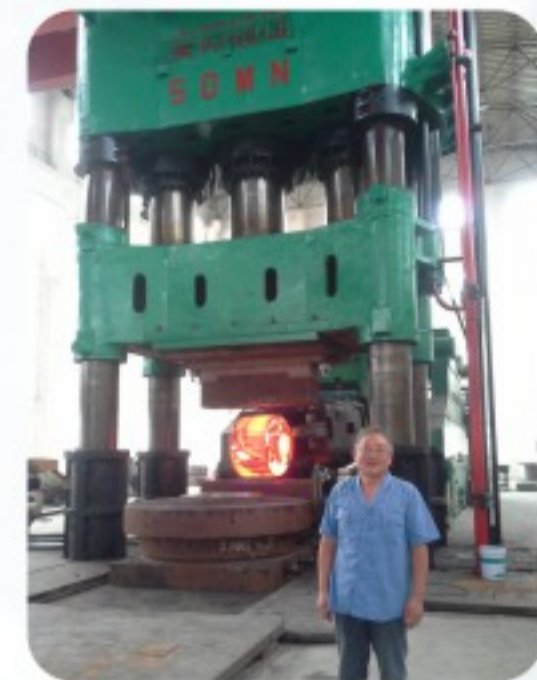
5000T自由锻液压机在鞍山客户 5000T hydraulic open die forging press in Anshan
