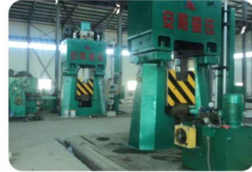
25KJ、31.5KJ、50KJ等6台 数控锤锻造汽车连杆 25KJ、31.5KJ、50KJ etc 6 sets of CNC hammer forge connecting rod
