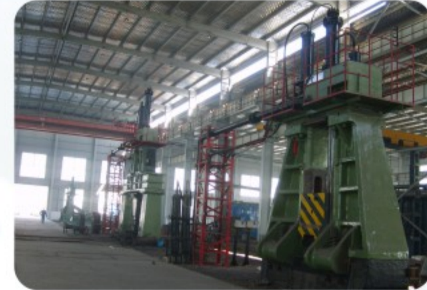
10T电液模锻锤和8T自由锻电液锤锻造煤机配件 10T hydraulic closed die hammer and 8T open die hammer forge part for coal machine
