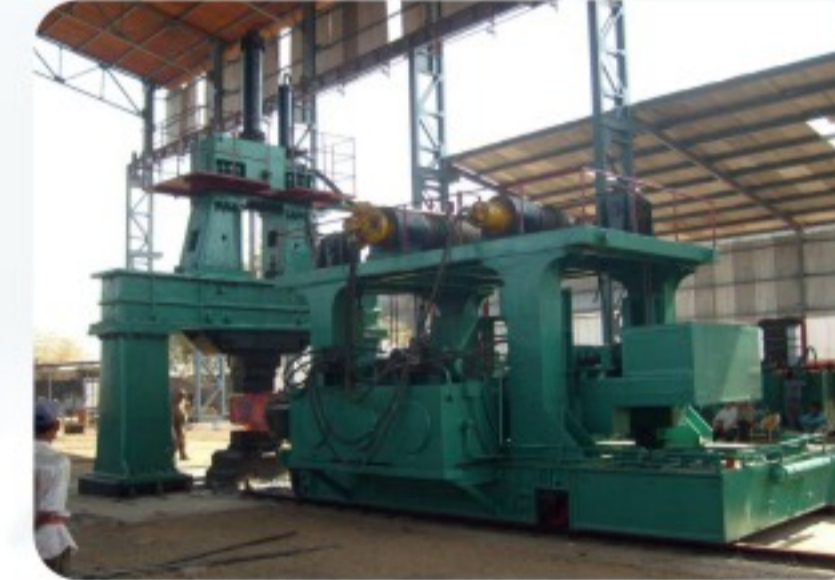
6T自由电液锤和8T锻造操作机在印度 6T hydraulic open die forging hammer&8T manipulator in India
