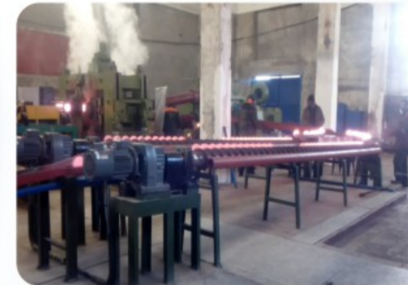
ZQ-120钢球斜轧机生产线在亚美尼亚 ZQ-120 skew rolling mill line produce grinding balls in Armenia
