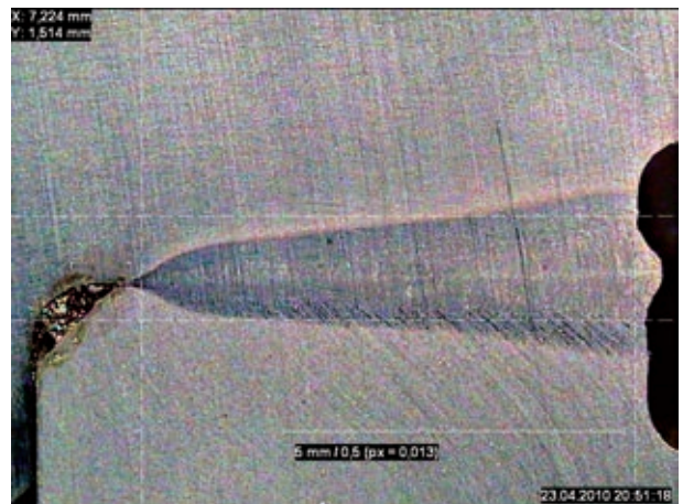
Cross section for the assessment of the welding seam quality.
