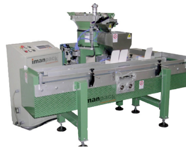
Weigh Scale especially designed for small counts and boxes under 5lbs. Good for screws, nails and assorted hardware.
