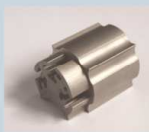
Material: SDK-11 Moly wire diameter: 0.18 Thickness: 30 Cutting times: 3 Roughness: 0.9
