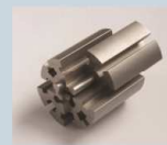
Material: SDK-11 Moly wire diameter: 0.18 Thickness: 40 Cutting times: 3 Roughness: 1.0
