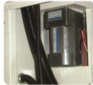
Z-axis up/down by motor
