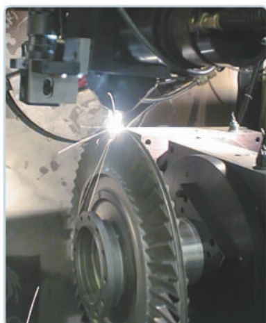
LENS Additive Repair
