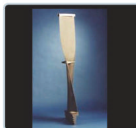
Compressor Blade Repaired by LENS System
