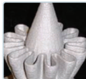
Exhaust Duct Fabricated by LENS System
