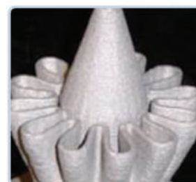
Exhaust Duct Fabricated by LENS System
