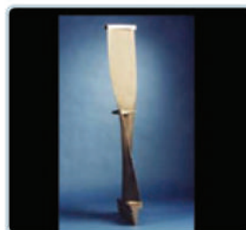
Compressor Blade Repaired by LENS System
