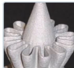
Exhaust Duct Fabricated by LENS System
