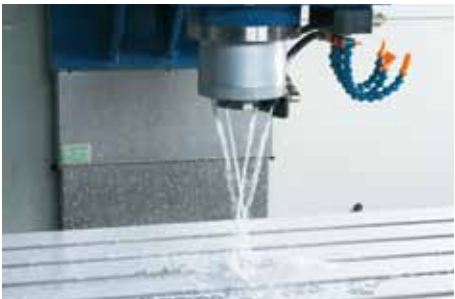
Coolants Jets Around Spindle Improved cooling efficiency on workpiece. (ISO 40 standard, ISO 50 optional)
