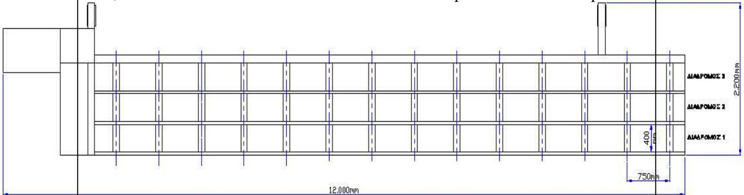
Over the corridors, there are braces that open-close with the aid of pneumatic pistons. The operator makes the selection via computer. This way, the -different length- cut rods are placed in a different corridor.
