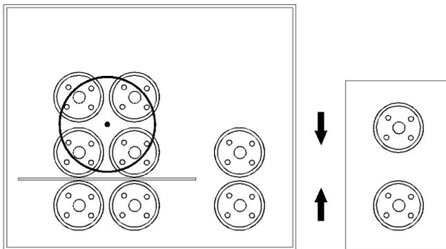
The free plastic rolls are installed upon a disk and have the ability to rotate. Two of those are placed opposite to metallic advance rolls and two ones remain inactive.
