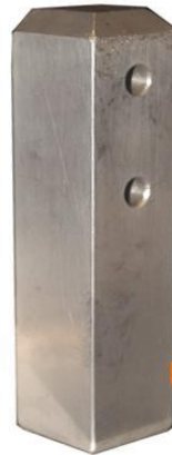
RB02 4 Holes altered to hold rest pad.
