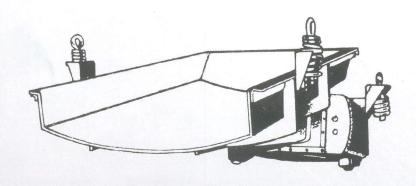
The feeder is an application of an Electro-Magnet to a suitable trough. Movement of the trough is obtained through a spring acted on by a powerful electro-magnet, working is synchronisation with the periodicity of supply. The positive through action induces flow with almost negligible friction between the material and the trough.
