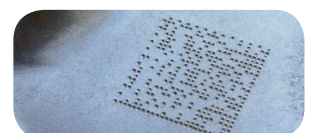
Datamatrix on Aluminium
