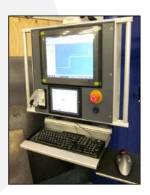
An optional additional panel PC can be used together with offline programming software.
