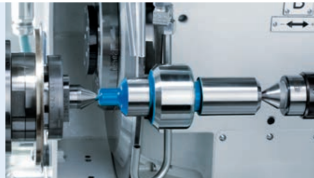
Workpiece clamped between centers - no need for a clamping chuck
