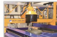
龙门切割头伴随移动集尘罩 Gantry cutting head with mobile dust cover
