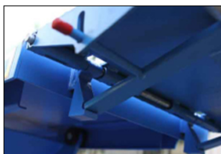
The strengthen extension slope can support the vechicle
