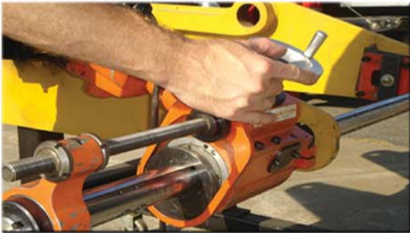
#2. Insert boring bar drive and motor
