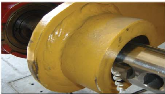
#3. Machine the bore to clean and prepare for welding
