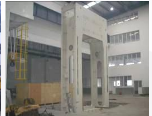
Discharge, transport and position the 126 ton presser frame
