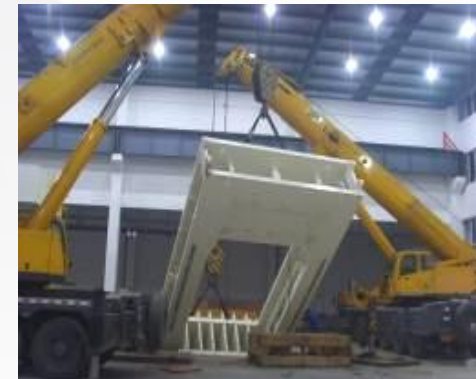
Discharge, transport and position the 126 ton presser frame
