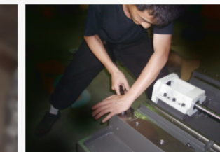
Carefully scraping on critical connection surfaces 重要結合面部位都需經過嚴密的銼花處理
