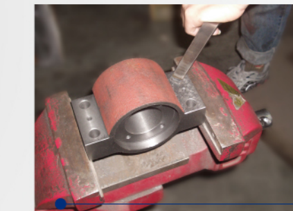
Carefully scraping on critical connection surfaces 重要結合面部位都需經過嚴密的銼花處理
