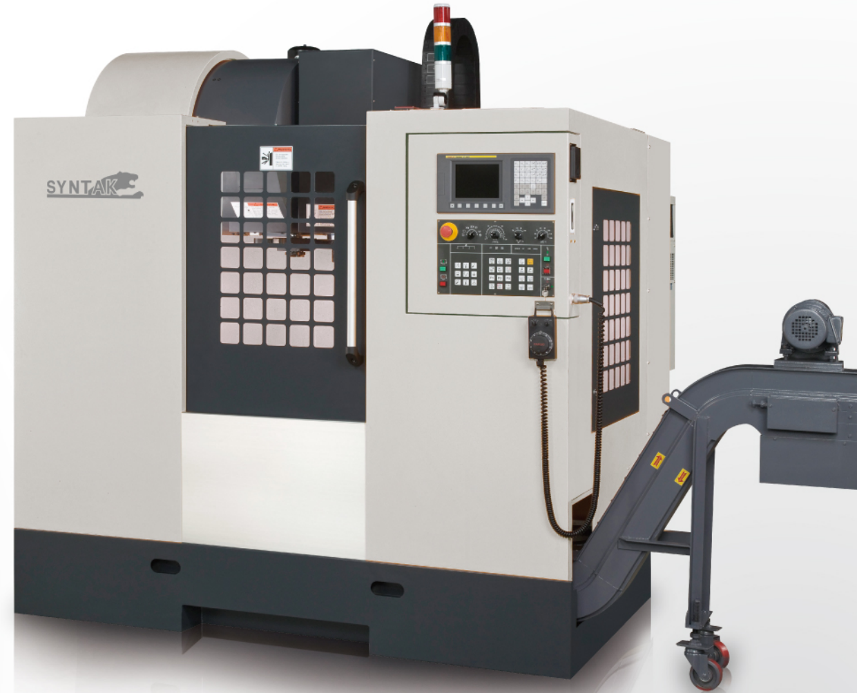
Chip conveyor can be loaded from either side 鐵屑輸送機能從機器之左邊或右邊安裝
