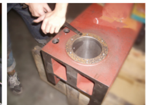
Carefully scraping on critical connection surfaces 重要結合面部位都需經過嚴密的銼花處理
