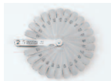
MFG-25-76 $17.08 25 blades, 12.7mm wide and 76mm long. Thickness (in millimeters) 0.04, 0.05, 0.06, 0.07, 0.08, 0.09, 0.10, 0.15, 0.20, 0.25, 0.30, 0.35, 0.40, 0.45, 0.50, 0.55, 0.60, 0.65, 0.70, 0.75, 0.80, 0.85, 0.90, 0.95, 1.00
