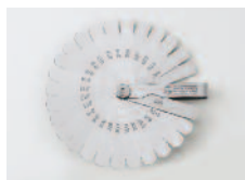
FG-25-3-SS $82.69 XF Series 25 stainless steel blades, 1/2" wide and 3" long. Thickness (in inches) .0015, .002, .0025, .003, .004, .005, .006, .007, .008, .009, .010, .011, .012, .013, .014, .015, .016, .017, .018, .019, .020, .021, .022, .023, .024, .025
