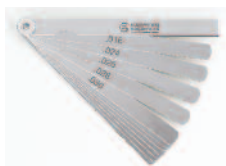
FG-26-6 $66.68 XF Series 26 blades, 1/2" wide tapered to 1/4" and 3" long. Thickness (in inches) .0015, .002, .0025, .003, .004, .005, .006, .007, .008, .009, .010, .011, .012, .013, .014, .015, .016, .018, .020, .022, .024, .026, .028, .030, .040, .060
