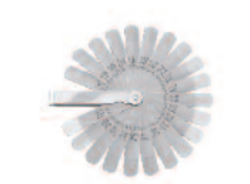
FG-22-STEP $31.13 22 blades, 1/2" wide and 3" long with .002 deep by 5/8" step ground at tip. Thickness (in inches) .004-.006, .005-.007, .006-.008, .007-.009, .008-.010, .009-.011, .010-.012, .011-.013, .012-.014, .013-.015, .014-.016, .015-.017, .016-.018, .017-.019, .018-.020, .019-.021, .020-.022, .021-.023, .022-.024, .023-.025, .024-.026, .025-.027
