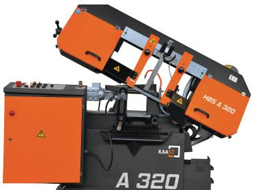
This new saw features a more rigid and compact design, automatic material feed, a parts counter and a built in coolant system. In keeping with an exceptionally high standard of machine quality, this KAAST saw incorporates infinitely variable band speed and cutting force for optimum cutting results.
