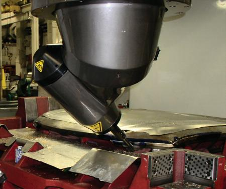
The PMT features a Direct Drive system which couples the large liquid cooled Torque Motor directly to the Ball-Nut for the absolute highest rigidity and response.
