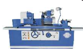
ABC- 1000mm X 150 CH HYDRAULIC CYLINDRICAL GRINDING MACHINE
