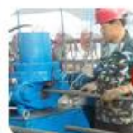
Upsetting of Steel Bar
