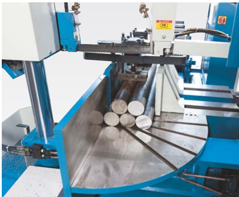
Both vises are designed as hydraulic bundle vises (standard equipment)
