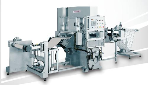
Hudson Cutting Solutions provides simple manual slide table feeds and a number of through-type mechanisms which continuously feed a variety of roll or sheet goods. Hardened and ground steel cutting plates are also available, along with linked mechanical low point stopping mechanisms to provide a kiss cutting capability. For applications more suited to soft matrix cutting, there are head mounted die holders and automatic pad shifter mechanisms.
