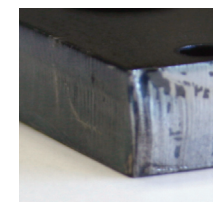
Conventional CO 2 Laser Cut Edge
