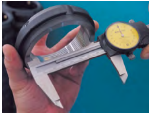
We measure the inner diameter of the locknut. (refer to photo)
