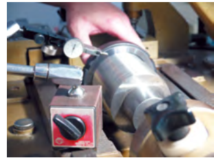
We measure the locknut thread run-out. (refer to photo)
