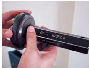
We check the thread precision by a gauge to insure ISO 4H. (refer to photo)
