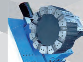
Baruffaldi TB400 Servo turret with polygon disc
