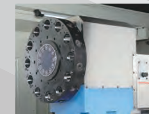
Baruffaldi TB Servo turret with VDI disc
