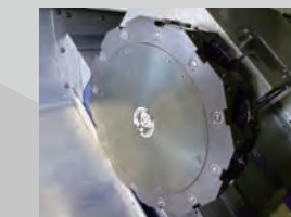
Baruffaldi TB power turret with BMT disc
