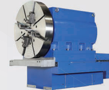
Tailstock with chuck & centre device for heavy parts cutting.
