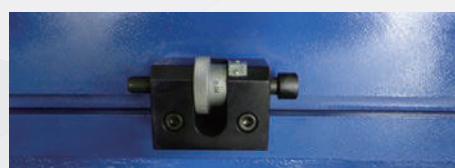
Micrometer Carriage Stop (Positioning system and auto power off)
