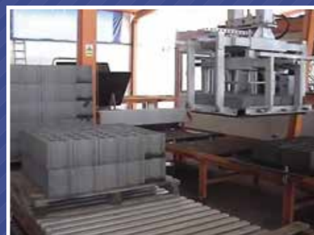
Lamellas is a conveyor for moving finished products for packing and moving to the warehouse
