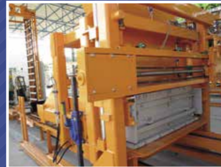
Facemix equipment for products with second layer
