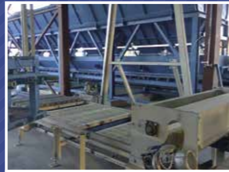
Rotating brush for wooden pallets cleaning
