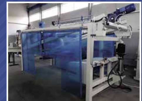
Equipment for decorative processing of surface of concrete products (paving stones, pedestrian blocks, etc.) with water supply under high pressure
