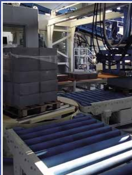
The packing machine for pallets with finished products
