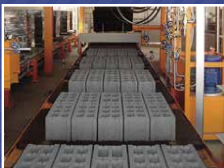
Pallet conveyor for transporting pallets with dry products to cubing station and after to pallet rotation - cross transport.
