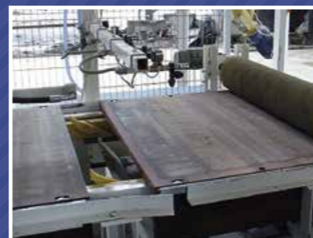
Device for spraying of working pallets
