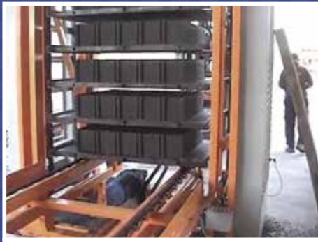
Elevator is an automatic device for accepting and raising pallets with fresh pieces – robot for putting pallets with fresh products into the curing rack (with 6-12 levels for blocks or the 2x 6-12 levels for paving stones)
