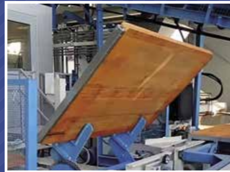
Pallet rotating device + cross pallet transport back to machine magazine, the pallets will be able to be used on both sides equally
