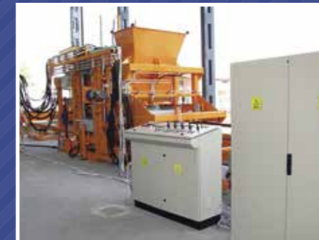
Automatic control system of the production line and the PC, Siemens computer program. Cables, system fuses, the alarm system security
