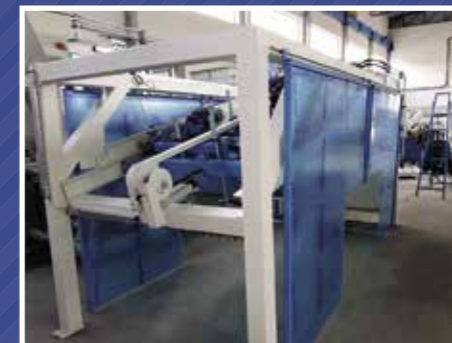
Equipment for decorative processing of surface of concrete products (paving stones, pedestrian blocks, etc.) with water supply under high pressure
