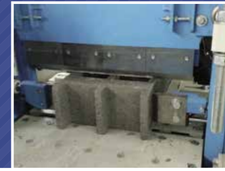
Splitter is a device for production of splitter blocks
