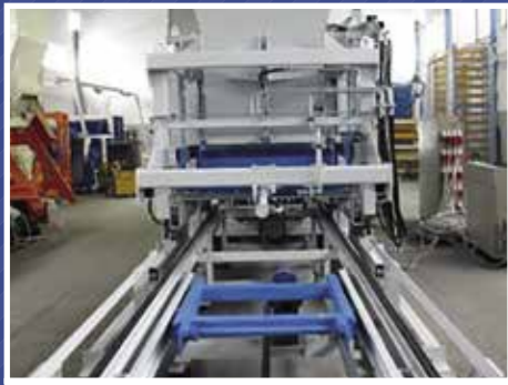
Transport of fresh concrete blocks from the machine with speed/start stop ramp regulation, consists of two chain transport systems
