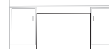
Knee Space Panel 35" high. Located at the rear of knee space areas.
