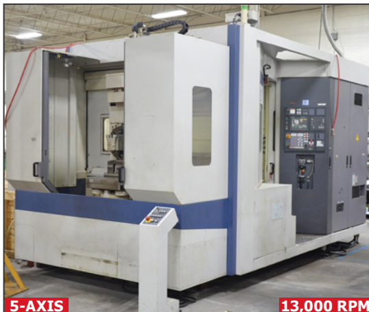
5-AXIS 13,000 RPM MORI SEIKI MH-630 5 axis CNC twin pallet horizontal machining center
