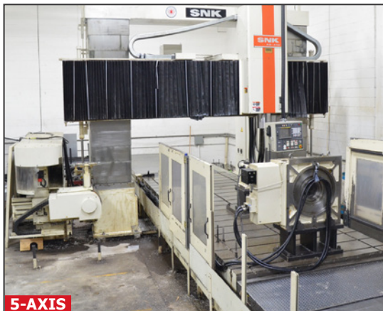
5-AXIS SNK RB-4NM double column 4 axis bridge type CNC machining center
