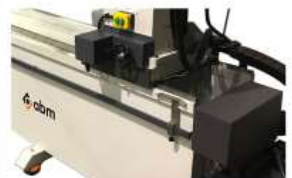
Automatic tilting option for magnetic bed - Automatic Infeed option by Motor control
