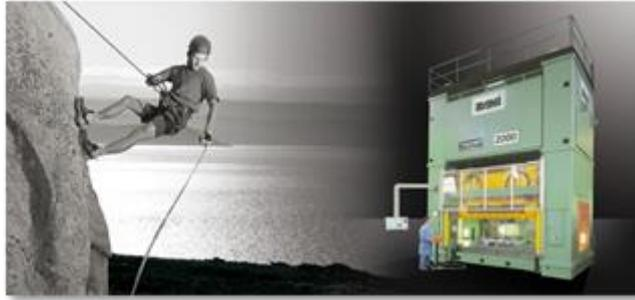
Our eccentric presses with capacity up to 630 Ton, 400 mm stroke length, and bolster up to 4000 mm
