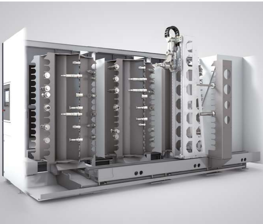
Tower magazine with storage capacity for 450 tools in the stage of extension.
