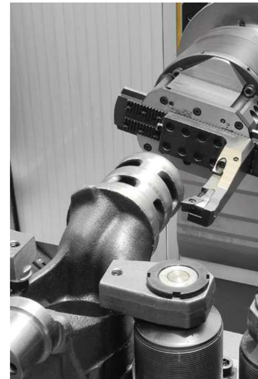
Flexible complete machining of different pivot housings for haulers on the Heckert HEC 500 Athletic with automatically exchangeable NC radial facing slide. Alternative solution with the advantage of reducing the processing time and the logistics expenses compared to machining on lathes.
