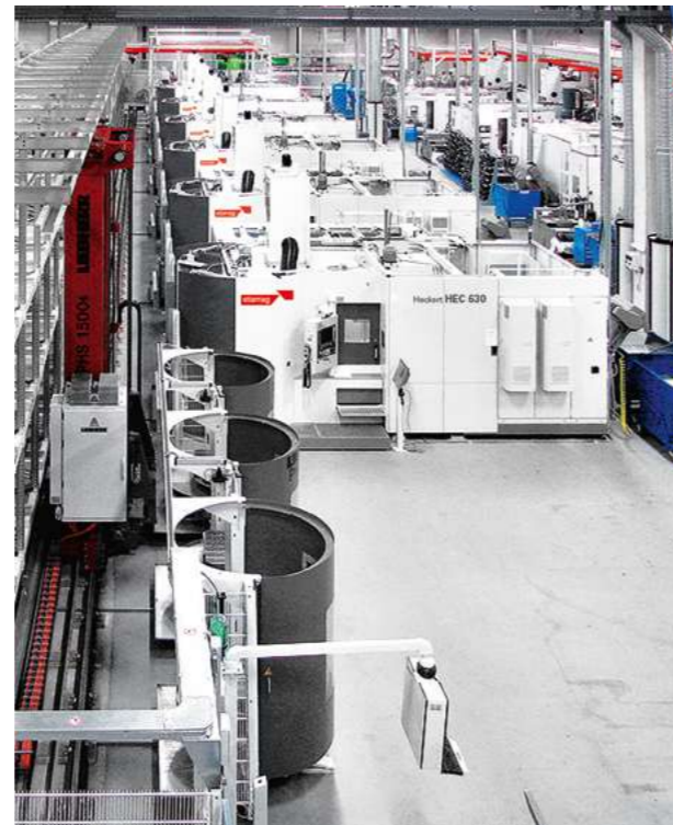
Flexible production system with 6 Machining Centers Heckert HEC 630 Athletic, pallet linear storage system and master control for for housing machining from batch size 1 up to large scale production.
