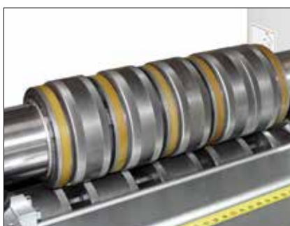
Rolls for standing seam and snap-lock seam.
