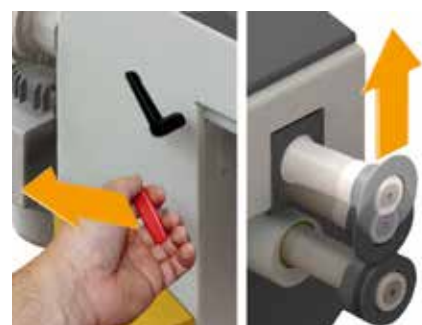
UnLock function opens the wheels immediately in an emergency.
