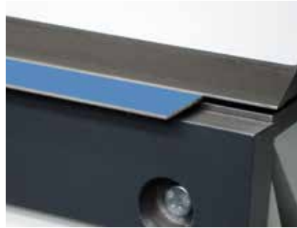
Automatic folding beam adjustment for thin and thick materials.
