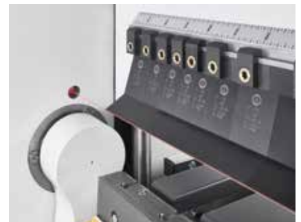
A laser automatically recognizes the exact tool height.
