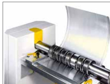
Rolls easily adjustable to the width of the part
