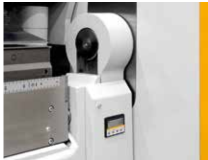
Optional digital display for folding beam adjustment.
