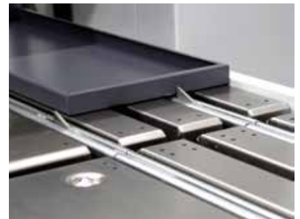
Parts aligned with the squaring arm.
