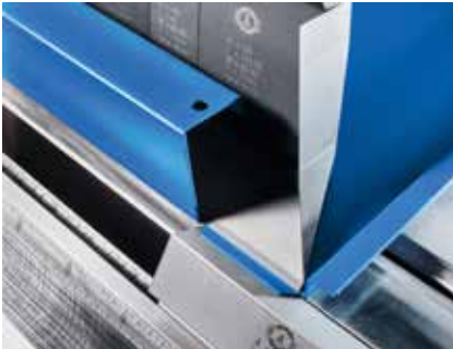
Bend tabs with segmented folding beam tools.
