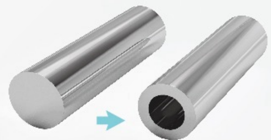
軸心孔位鑽孔 Center hole drilling
