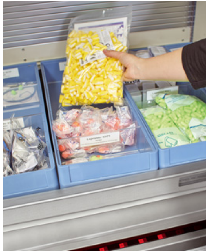
Hänel compartment and sub-level indicators show where the requested items are located
