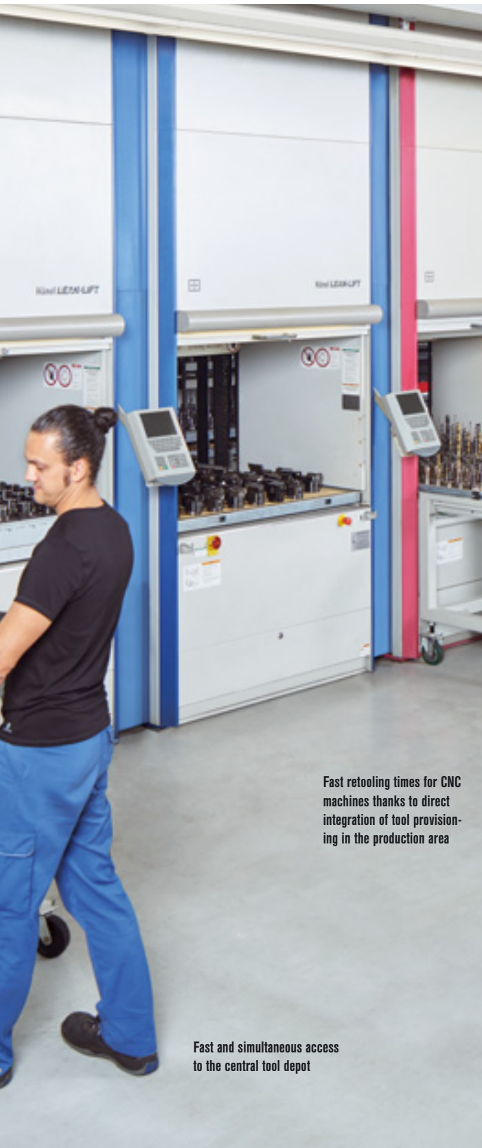
Height-optimized storage of various tools on the Hänel multifunction container
