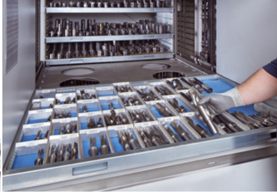
Height-optimized storage of various tools on the Hänel multifunction container
