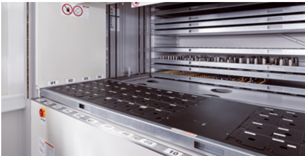
Individual containers in a Lean-Lift® system can be equipped with the VendiShelf system as required
