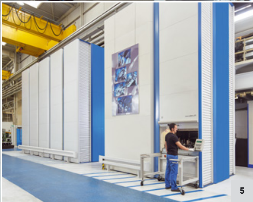
Fast retooling times for CNC machines thanks to direct integration of tool provision- ing in the production area
