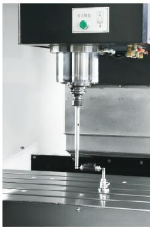
Spindle deflection detection
