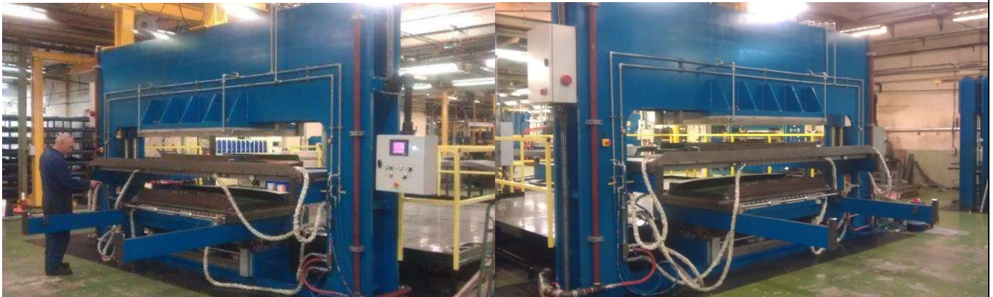
5000 kN Compression Hydraulic Press with double Daylight for Large Rubber Seals
