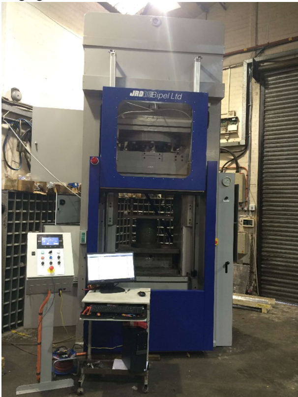
BIPEL 3000kN hydraulic press for composite metal forging
