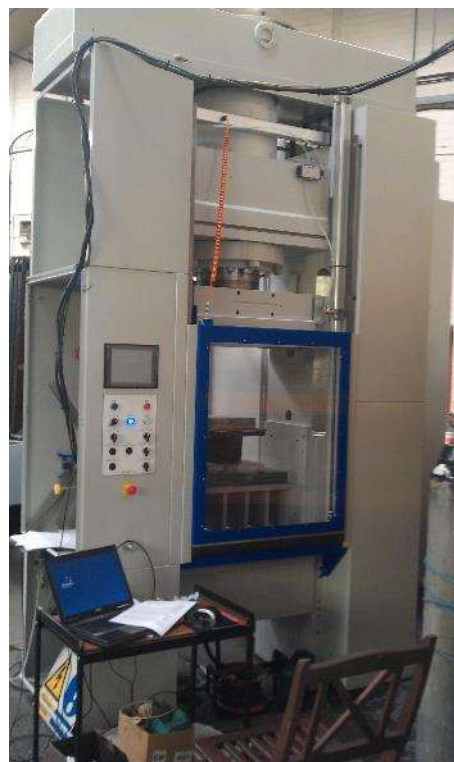
2000 kN Metal Powder Compaction Hydraulic Press
