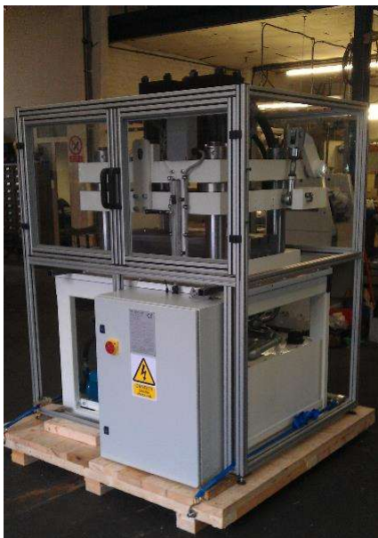
750 kN Hydraulic Cutting Press for the Medical Industry
