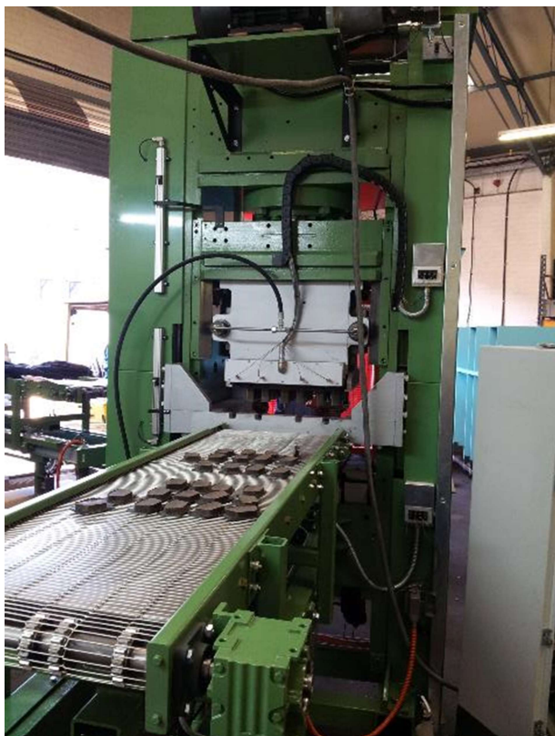
1500 kN Silicon Sheet Moulding Hydraulic Press
