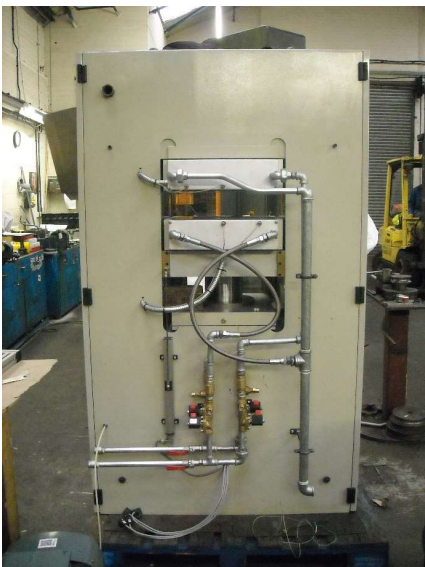
500 kN Laboratory Heating and Cooling Hydraulic Press for High Temperature Material Moulding at 450°C
