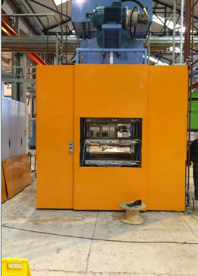
10000 kN BIPEL Hydraulic Press for High Density Carbon Fibre Moulding
