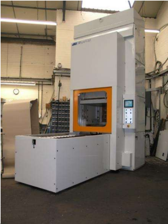
5000 kN Compression Hydraulic Press with double Daylight for Large Rubber Seals
