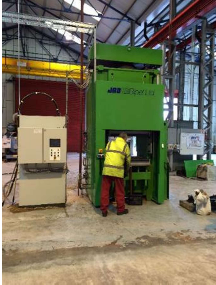
4500 kN BIPEL Hydraulic Press for High Density Carbon Fibre Moulding
