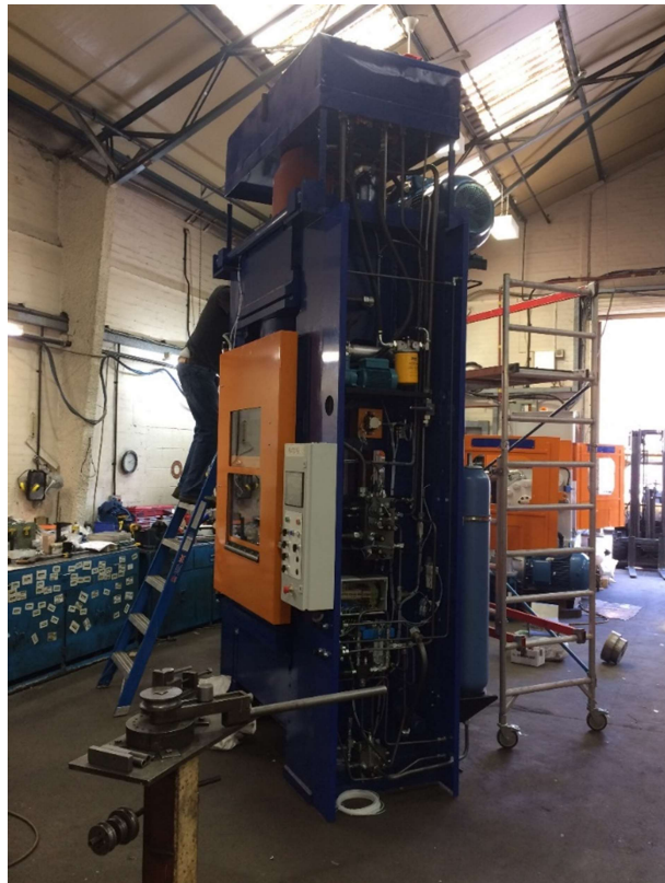
BIPEL 3000kN hydraulic press for metal drawing
