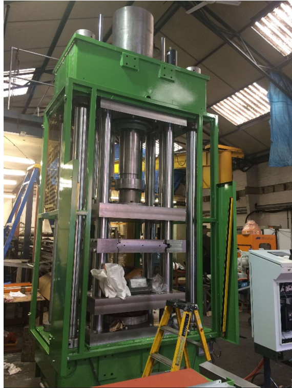
Re-engineered four column press for metal forming Fitted with two cylinders
