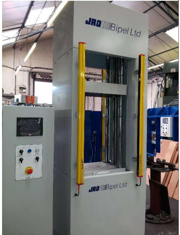
1000 kN Hot Clamping Press for Carbon Fibre Tube
