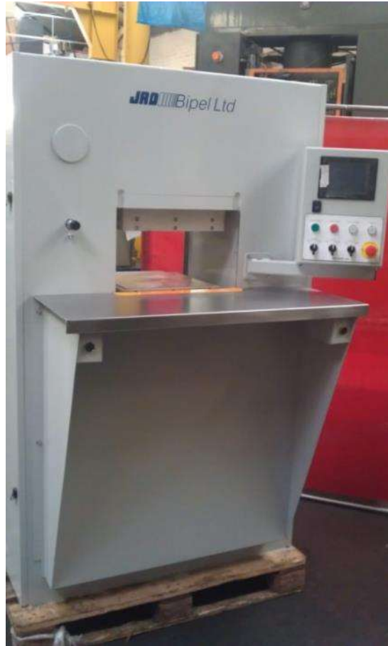
1200 kN Compression Moulding Press for the Automotive Industry
