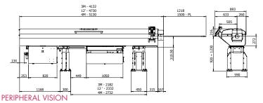
Barstock Straightness Specifications and Performance For optimum rotational performance speeds, bar stock straightness needs to be .020" per 3.25 feet, non accumulative. Bar stock out of this tolerance will not run at optimum RPM. Other factors such as material type (brass, copper, bronze and other malleable materials), clamping efficiency of the machine workholding, alignment of the bar feed, oil type, bar preparation and spindle liners will affect optimum RPM capability of the system.
