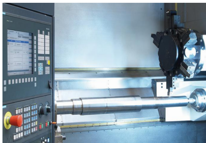
Work zone: upper tool turret
