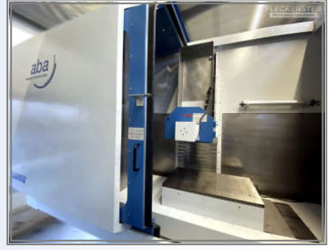
1559 ABA POWERLINE 1006 CNC (retrofit 2022) SINUMERIK 840 D, grinding area 1.000 x 600 mm, cross travel (Z-axis) 540 mm, vertical travel (Y-axis) 500 mm, grinding spindle 18,5 kW, grinding spindle 1.000 - 2.600 min-1
