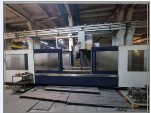
1634 SORALUCE TA 35 (2011) HEIDENHAIN iTNC 530, X-Y-Z 3.500x 1.250x1.000 mm, 24 kW, 3.000 rpm, ATC
