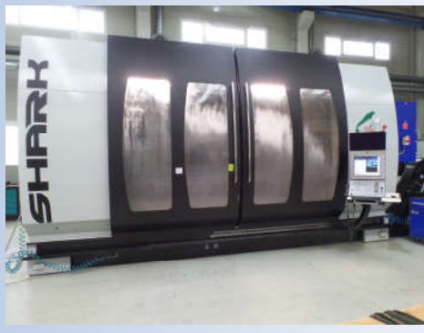
1592 PARPAS SHARK One (2016) HEIDENHAIN iTNC 530 HSCI, X-Y-Z 3.500x1.050x1.200 mm, clamping table 4.000x1.000 mm, 2-axis milling head 29 kW, 0-18.000 min-1m HSK 63A-DIN 69893, 30-fold ATC, tool Ø 90 mm
