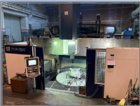
1631 DANOBAT VTC 2800 (2010), SINUMERIK 840 D, indexable crossbeam, max. swing 2.800 mm, table Ø 2.400 mm, max turning height 2.000 mm, ATC 20, C-Axis, straight and angular milling head, grinding option
