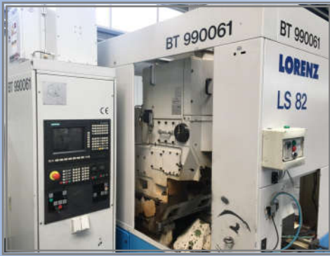
1554 LORENZ LS 82 (1999), SINUMERIK 840 C, workpiece external Ø 80 mm, stroke range 250—1.500 DH/ min, max. stroke length 55 mm, max. tool Ø 180 mm
