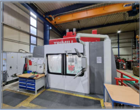
1630 TRIMILL VF3016 (2017) HEIDENHAIN iTNC 530 HSCI, X-Y-Z 3.000 x 1.600 x 1.200 mm, B+C axis, table 3.500 x 1.750 mm, 2-axis fork milling head T21C, 10-24.000 min-1, 42 kW, HSK-A 63, 50-fold tool changer ,
