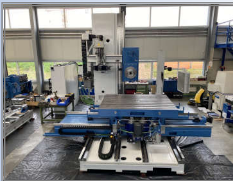
1610 UNION TC 130 (2004/2022) HEIDENHAIN iTNC 530 , X-Y-Z-W 2.500x2.000x1.500x750 mm, quill Ø 130 mm, ISO 50, 3.000 rpm, b-axis 360°. 40 ATC , nc rotary table 1.600 x 2.000 mm, 3-min 6.000 mm/min
