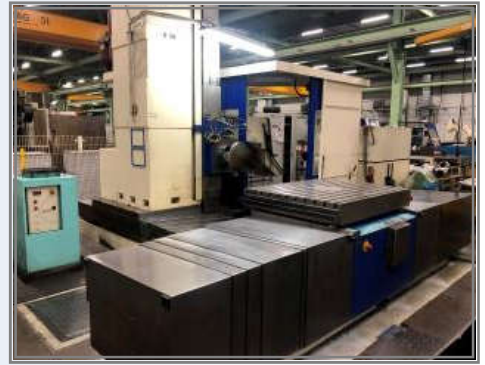
1596 CASTEL GREEN (1993) HEIDENHAIN TNC 155, X-Y-Z-W 3150x1300x1050x470 mm, rotary table load 10 to., table size 1.200 x 1.500 mm
