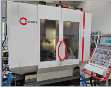
1636 HERMLE C40U dynamic (2003) HEIDENHAIN iTNC 530, X-Y-Z 850x700x500 mm, nc-rotary table Ø 800 mm, ATC 38, 28.000 rpm, Capto C5
