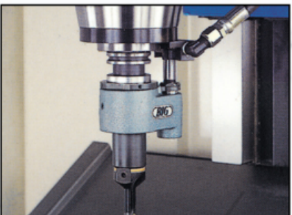
Coolant through tool
