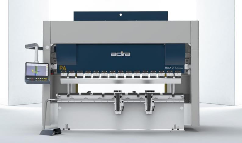
The HEXA-C® frame ensures better bending precision, given that the movable ram stays perfectly aligned with the fixed ram.
