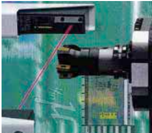
Automatic tool length measurement protector.
