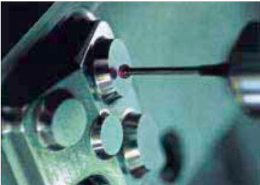
Automatic workpiece measurement.
