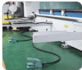
▲ Laser light curtain safety system 雷射光幕保護
