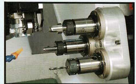
Precision flexible transfer machines equipped with 3-tool 4-axis Multi-Process Modules (patented) with tool change time in less than 0.4 seconds (chip to chip)
