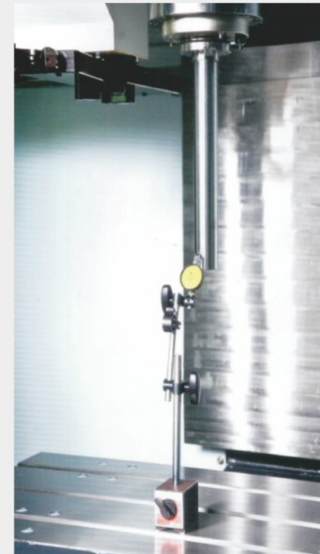
▲ 主轴检测棒检验 Inspection of spindle check rod
