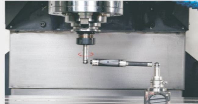
球杆仪真圆度检测 True roundness measurement of ball instrument
